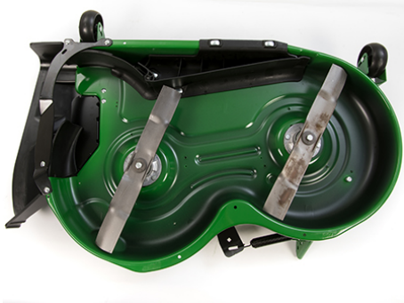
42A Mower underside (shown with optional MulchControl)
