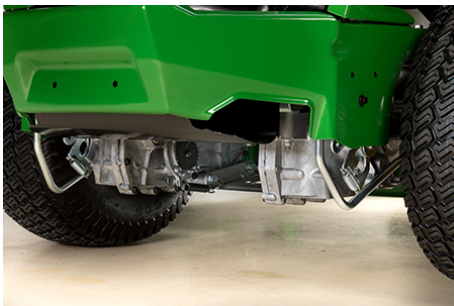
Hydrostatic transmissions set low in vehicle
