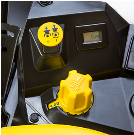
Mower deck lift/cut-height adjustment
