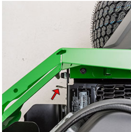
Tow-valve control (left side shown)
