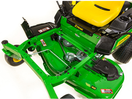
U.S. Z325E with foot platform removed to show frame
