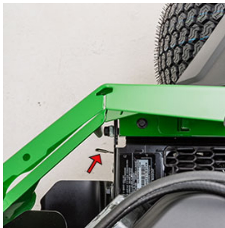
Tow-valve control (left side shown)
