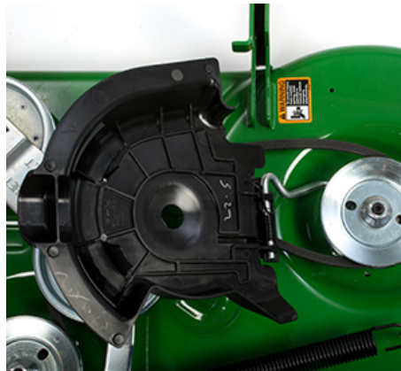
Flip-up cover for easy spindle-pocket access
