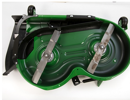
MulchControl baffle closed
