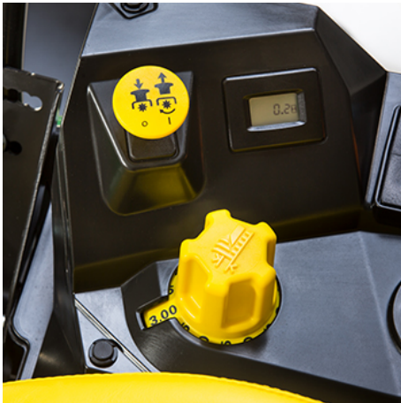
Mower deck lift/cut-height adjustment
