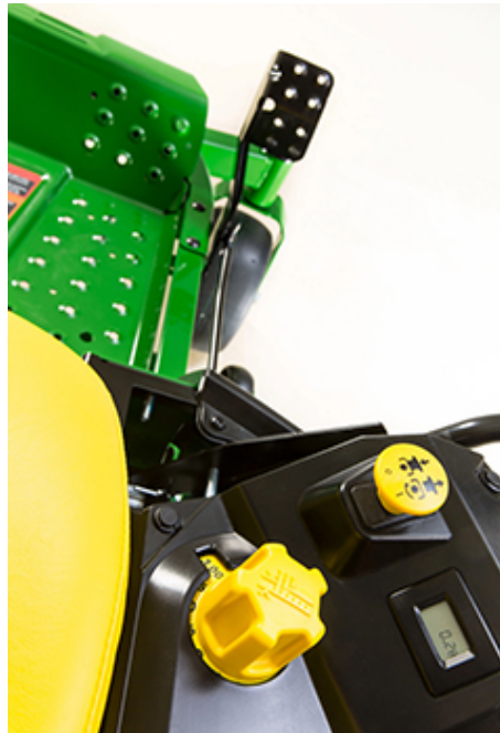
Foot pedal lift and cut-height adjustment
