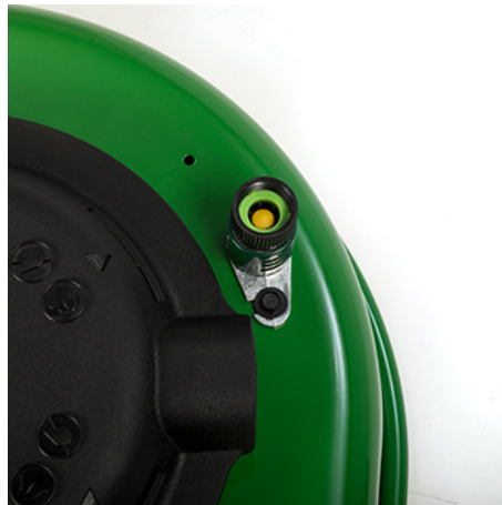
Mower wash port with locally purchased hose connector
