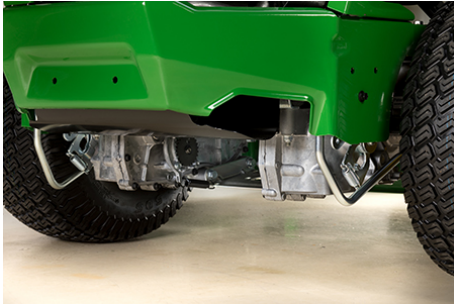
Hydrostatic transmissions set low in vehicle
