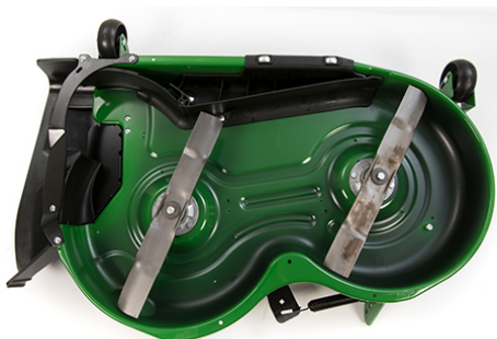
MulchControl baffle open
