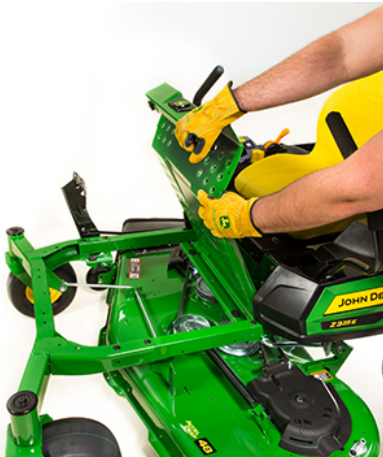
Footrest is easily removed for easy access to mower
