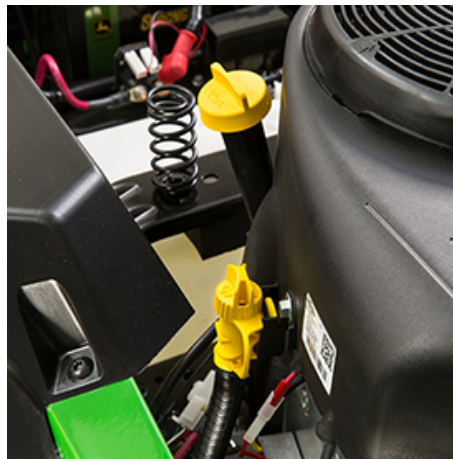
Engine oil check/fill tube and oil-drain tube
