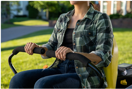
Motion-control levers in operating position disengages park brake
