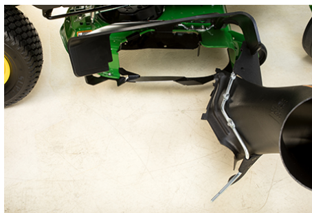
Rear MulchControl baffle removed to allow for chute installation
