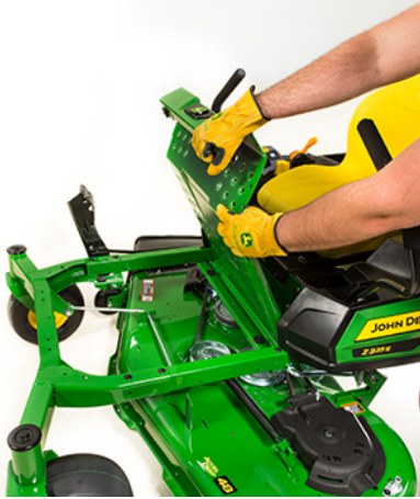
Footrest is easily removed for easy access to mower
