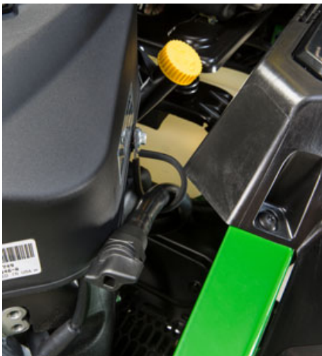
Engine oil check/fill tube and oil-drain tube
