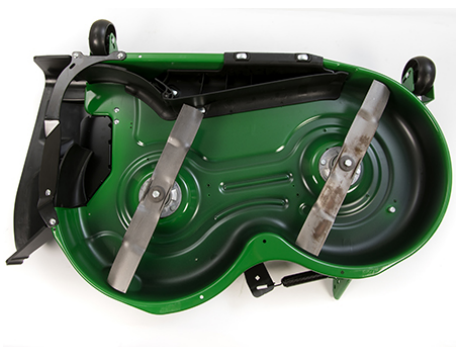
MulchControl baffle open
