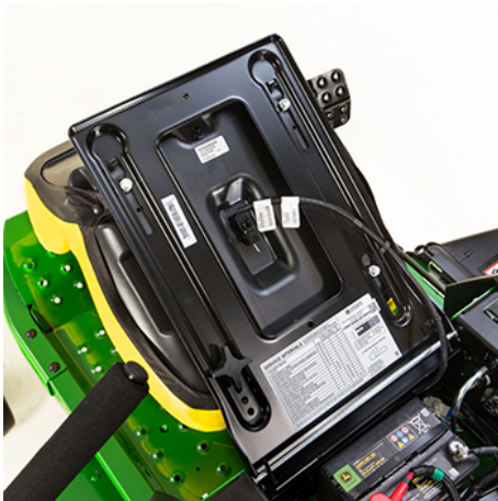
Interlock switch is located under the seat
