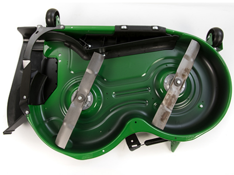
42A Mower underside (shown with optional MulchControl)
