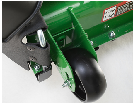
Mower wheels are double captured
