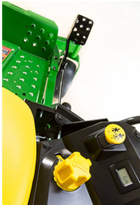
Foot pedal lift and cut-height adjustment
